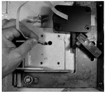
Once you've made sure the wire cable is not crimped or in contact with any sharp surface, attach the lock to the safe's mounting plate. Use the four  $\frac{1}{4}$ -20 (or metric M6) screws provided. Tighten securely so the lock is attached firmly to the plate.
